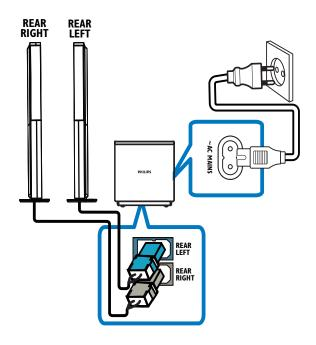
Connect the rear left and rear right speakers to the matching connectors at the bottom of the wireless receiver. For RWSS9500
